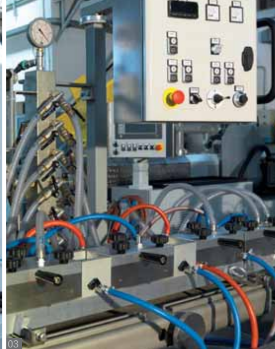
01. traino haul-off unit - 02. taglierina cutting unit - 03. calibratore calibrating table
